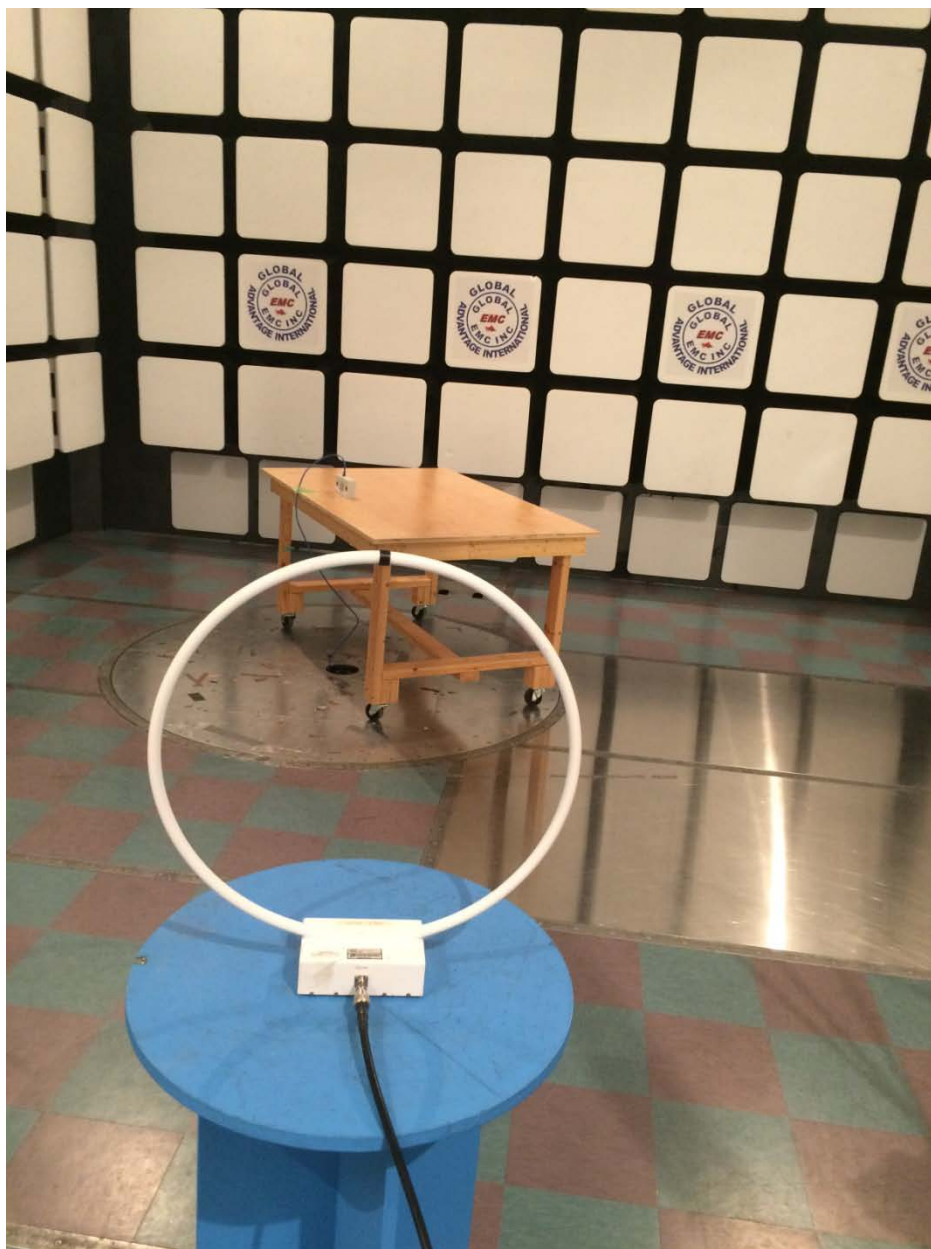
Figure 1: Radiated emission setup – photo 1
