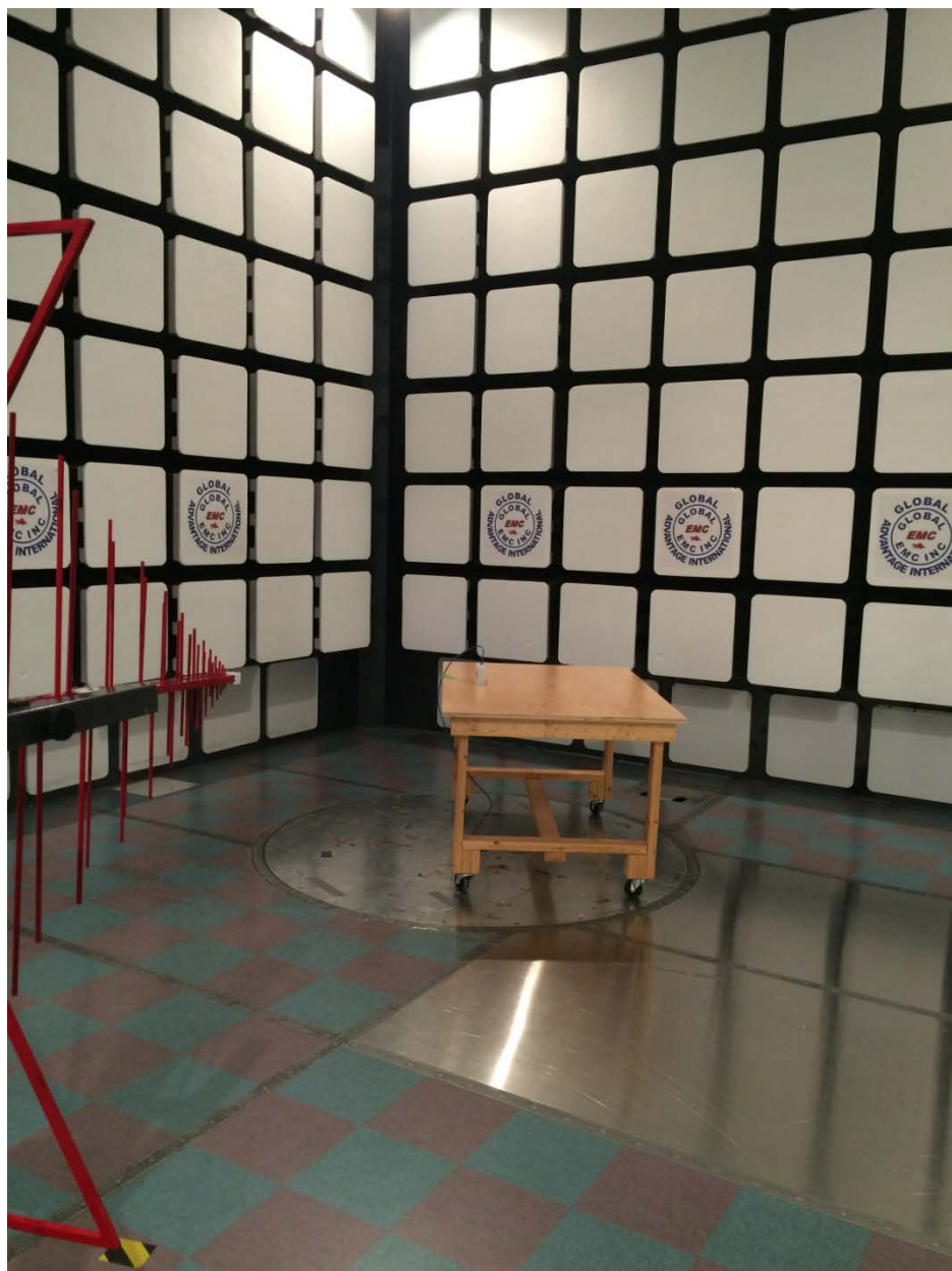
Figure 2: Radiated emission setup – photo 2
