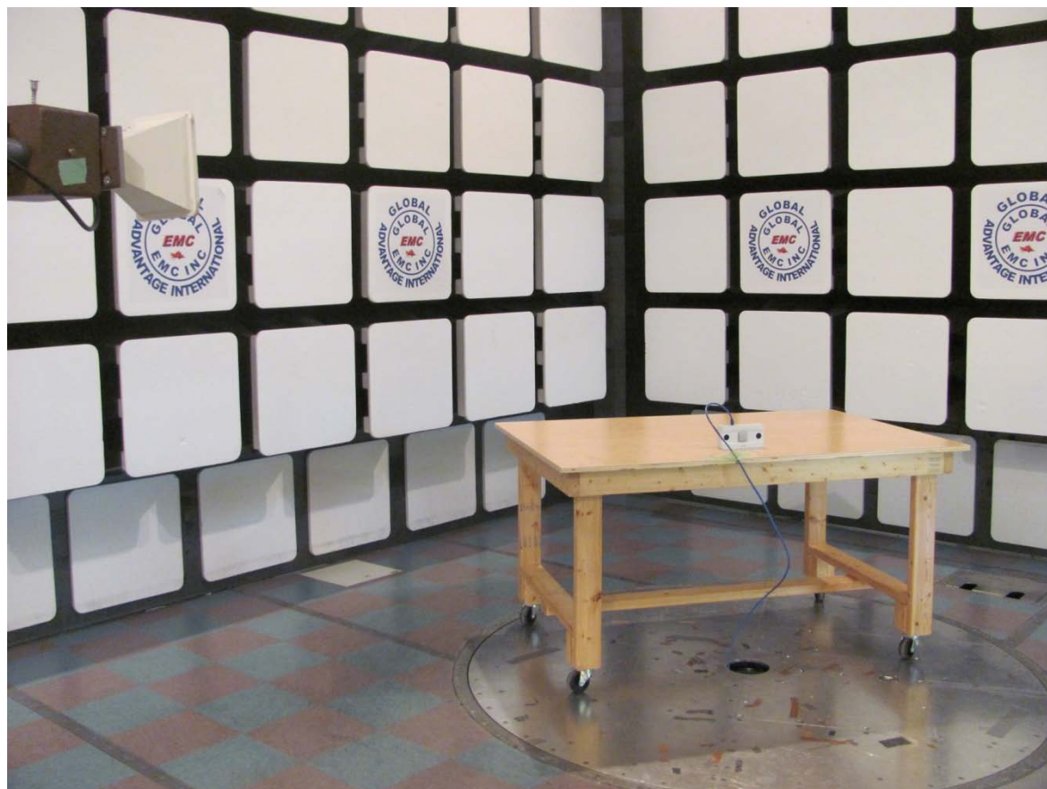
Figure 3: Radiated emission setup – photo 3
