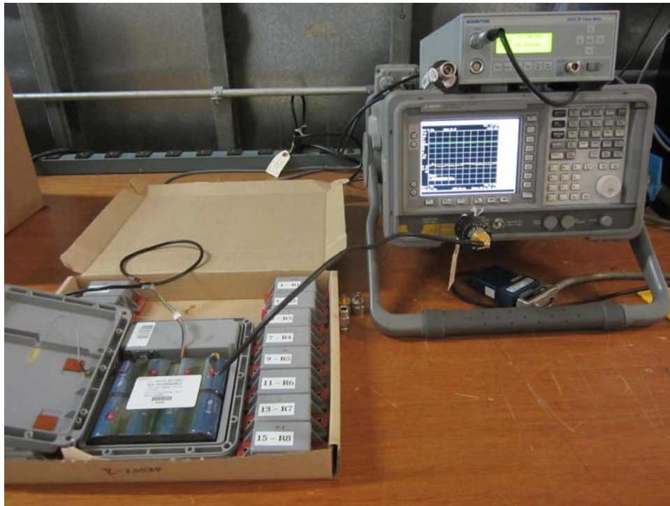
Peak Conducted Output Power / Test Setup
