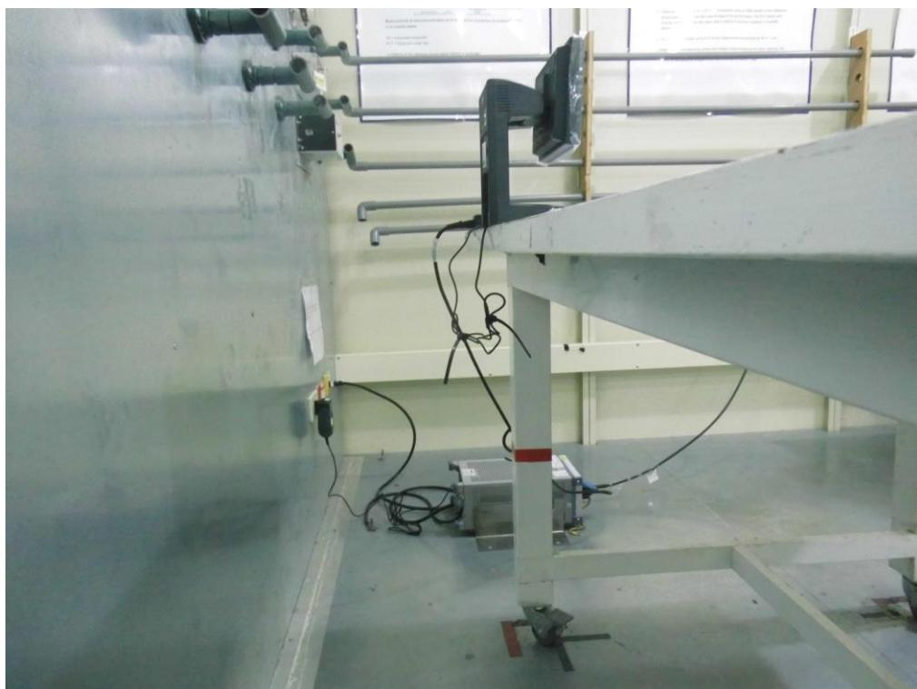
**Radiated emission test photos**
