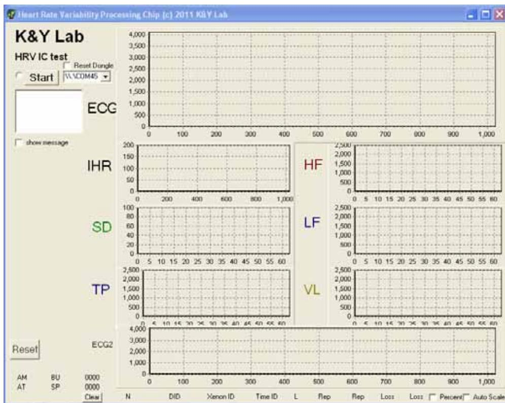
View receiver data(ECG waveform, HR, HRV index)
