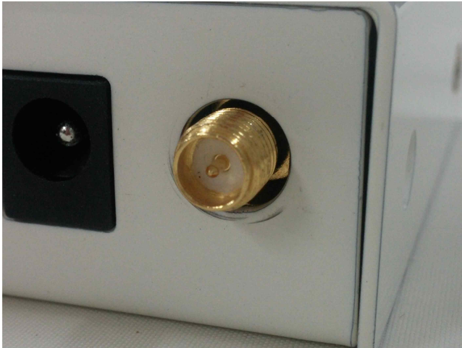
male type pin connector
