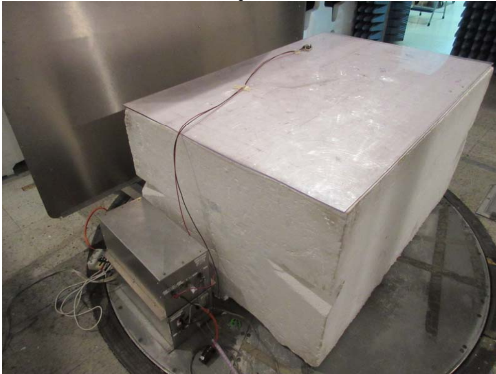
Test Setup for Conducted Emissions
