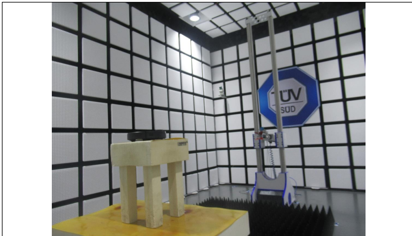
Radiated Emission test (1000MHz to 18000MHz)
