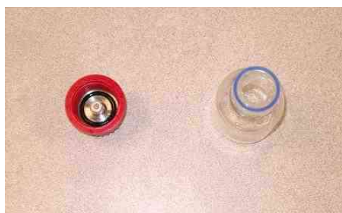
Figure 18 - Open coaxial probe with the bottle cap
