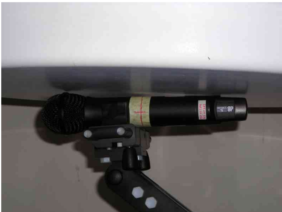
Figure 10 – Tested device position: with the Left side against the phantom
