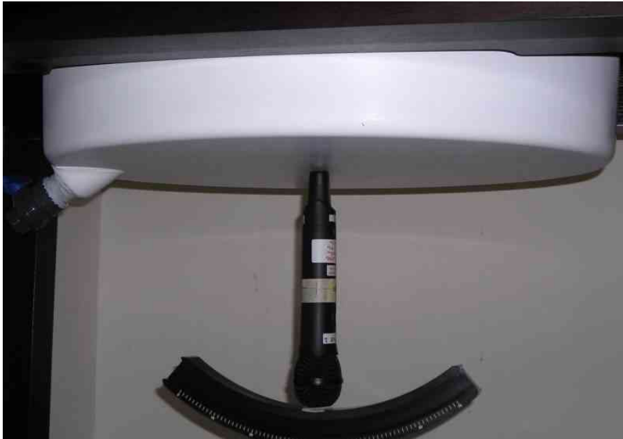
Figure 11 – Tested device position: with the Bottom against the phantom
