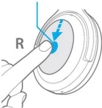
Slowly swipe up from the bottom edge to the center, and **HOLD** your finger at the center of the earcup until the desired volume level is reached
