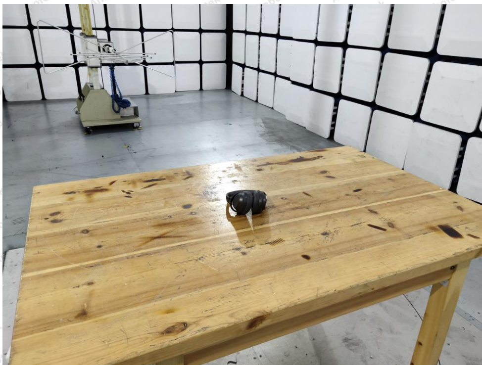
Photo of Radiation Emission Test
