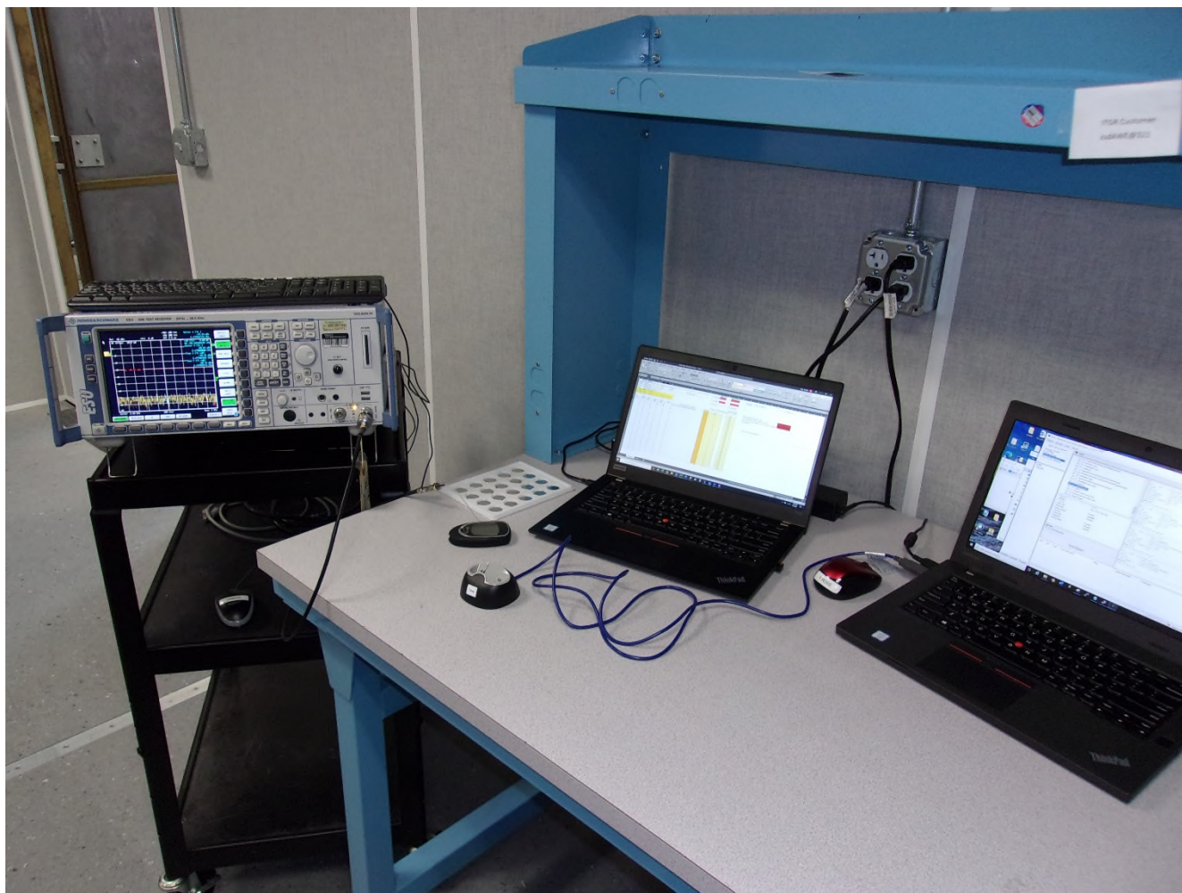
Photo 1.2-1 – Conducted Test Setup
