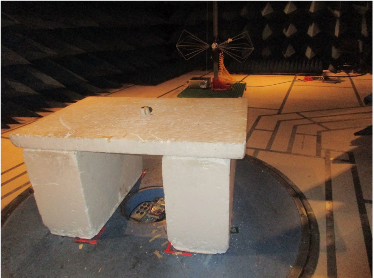
Figure 3: Radiated Emissions – Back View - 30 MHz - 200 MHz - EUT on Side
