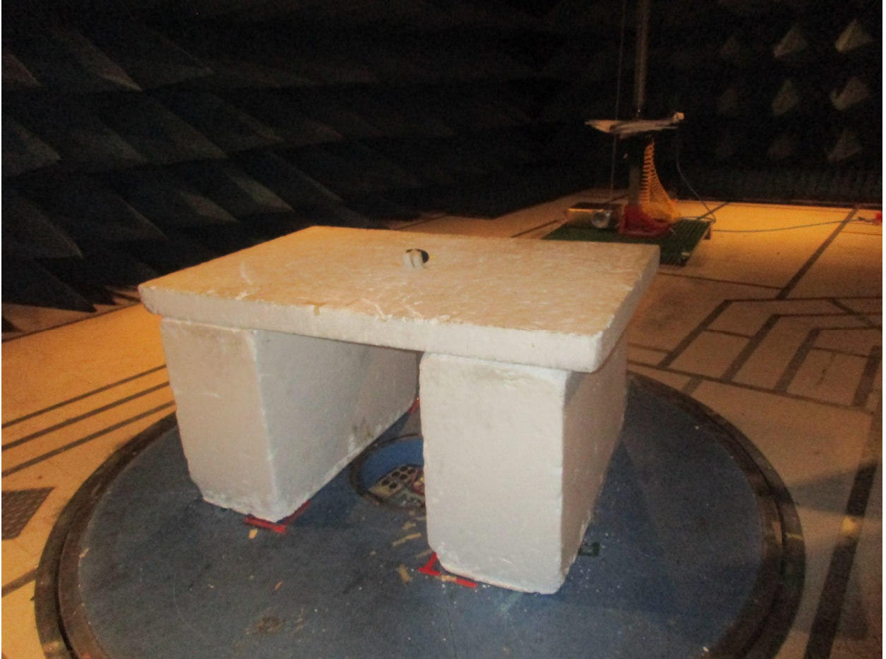
Figure 4: Radiated Emissions – Back View - 200 MHz - 1 GHz - EUT on Side
