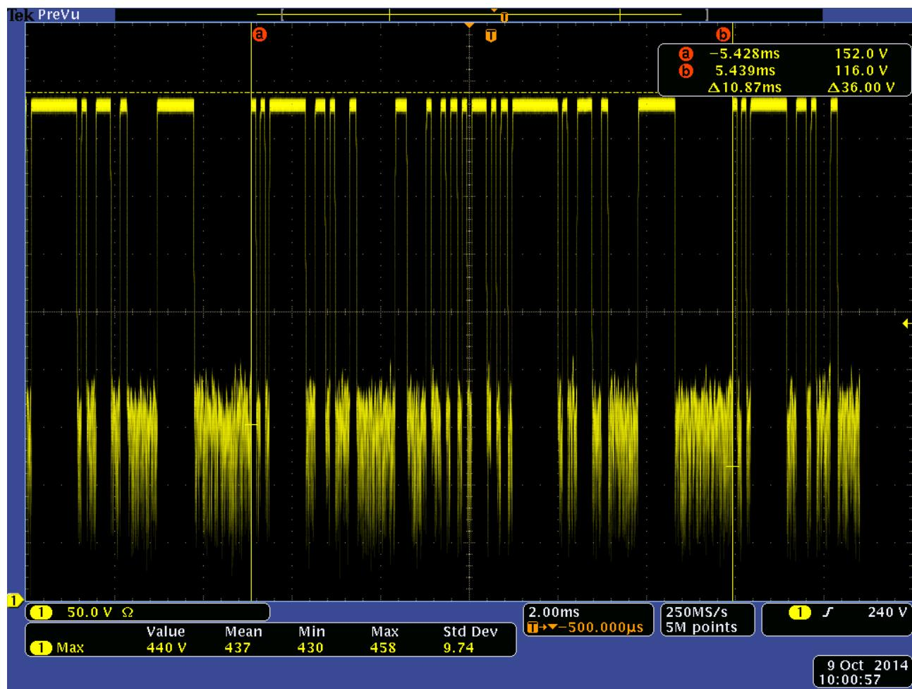
Total Pulse Time with Blanking Interval is 10.87 ms
