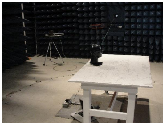
FIGURE 2: RE Test Setup - Active Loop Antenna Vertical and Horizontal Polarization
