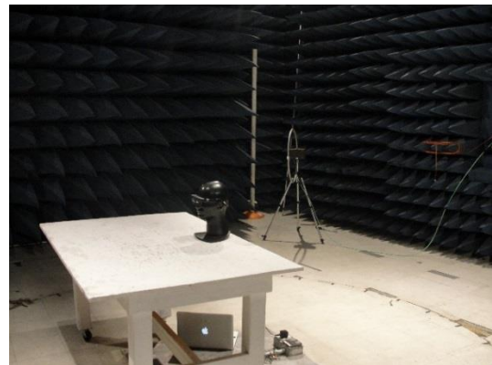
FIGURE 2: RE Test Setup - Active Loop Antenna Vertical and Horizontal Polarization
