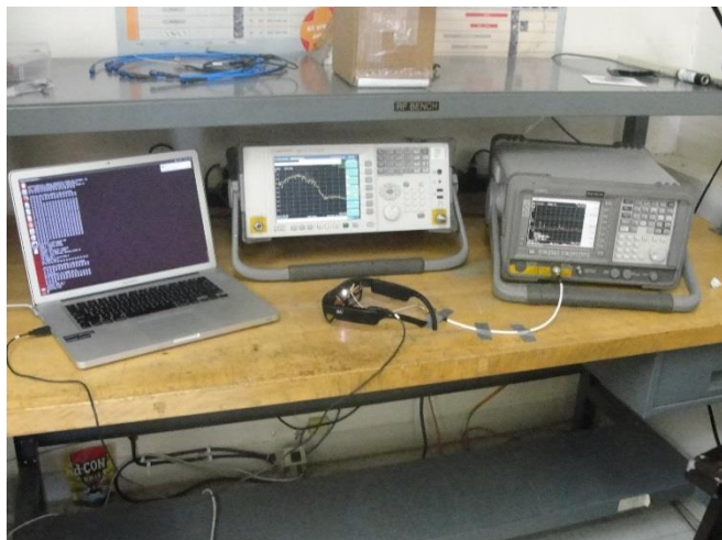
Figure1: Conducted RF Test Setup
