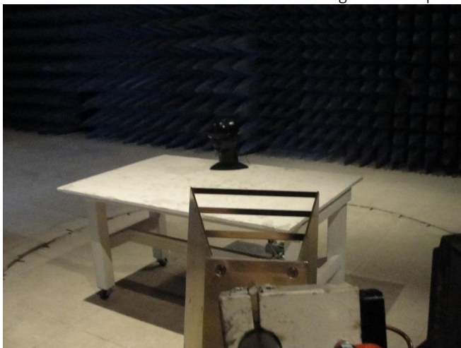
Figure 10: RE Test Setup DRG Horn Antenna(1-18GHz)
