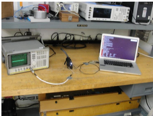
Figure 6: Conducted Spurious Emissions Test Setup For frequencies >26.5 GHz
