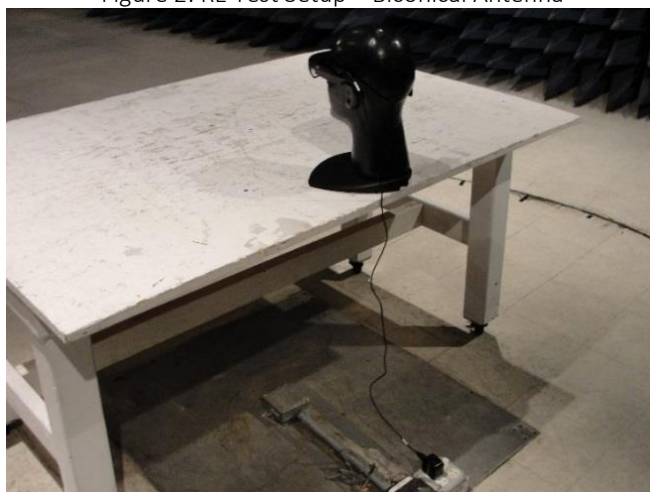
Figure 4: EUT RE Test Setup
