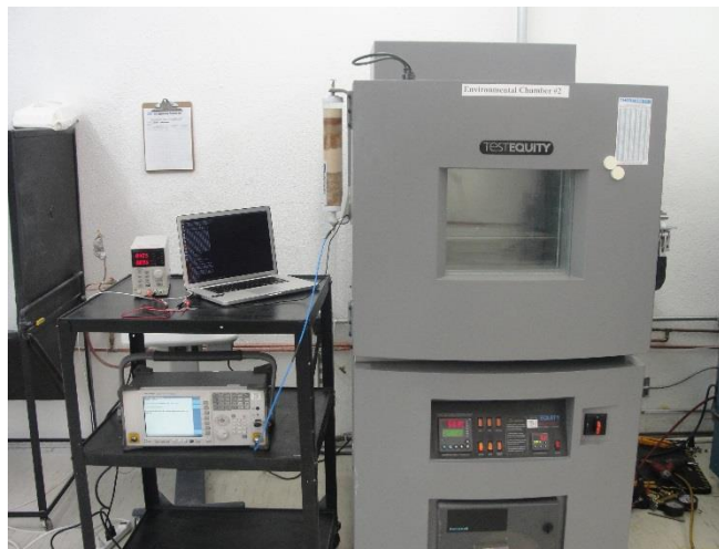
Figure 9: Frequency Stability Test Setup
