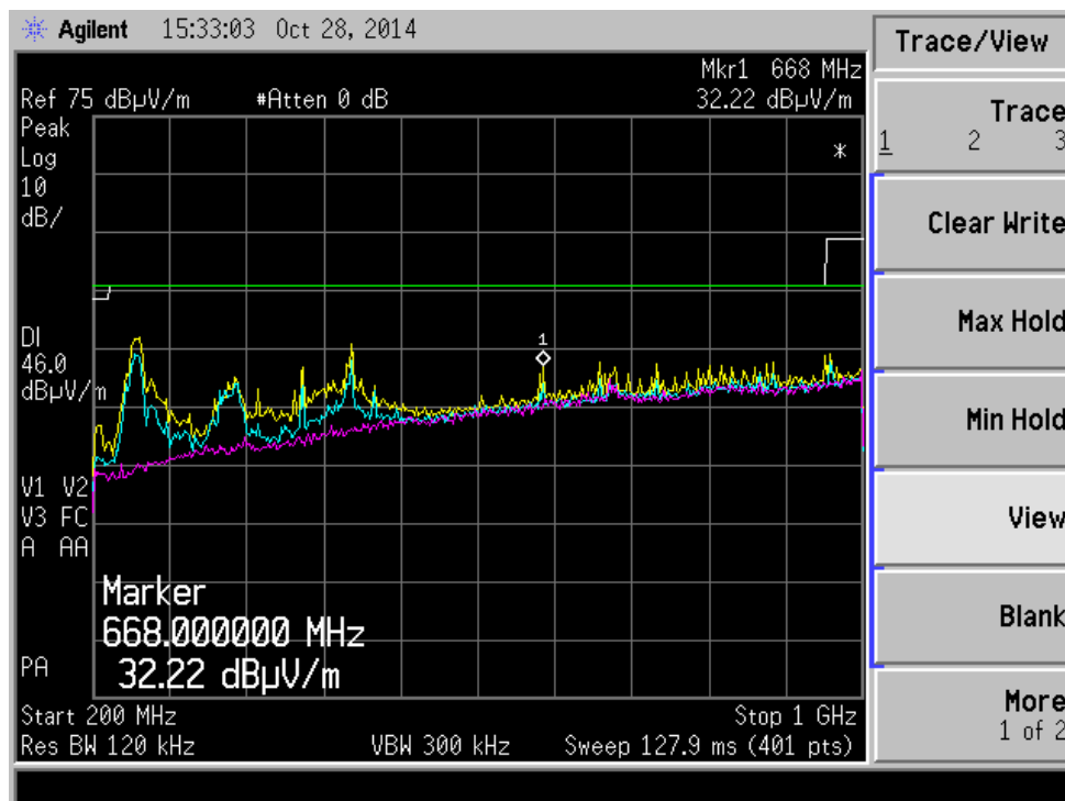
FIGURE 51: Log-Periodic, Horizontal Polarization: 802.11 & BT Blue trace – EUT off, Yellow trace – EUT on, Magenta – chamber background
