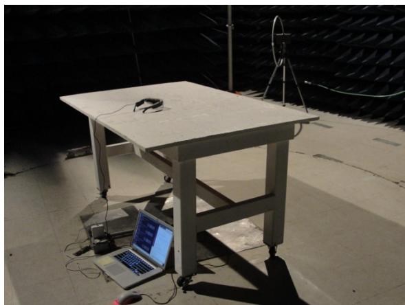
FIGURE 2: RE Test Setup - Active Loop Antenna
