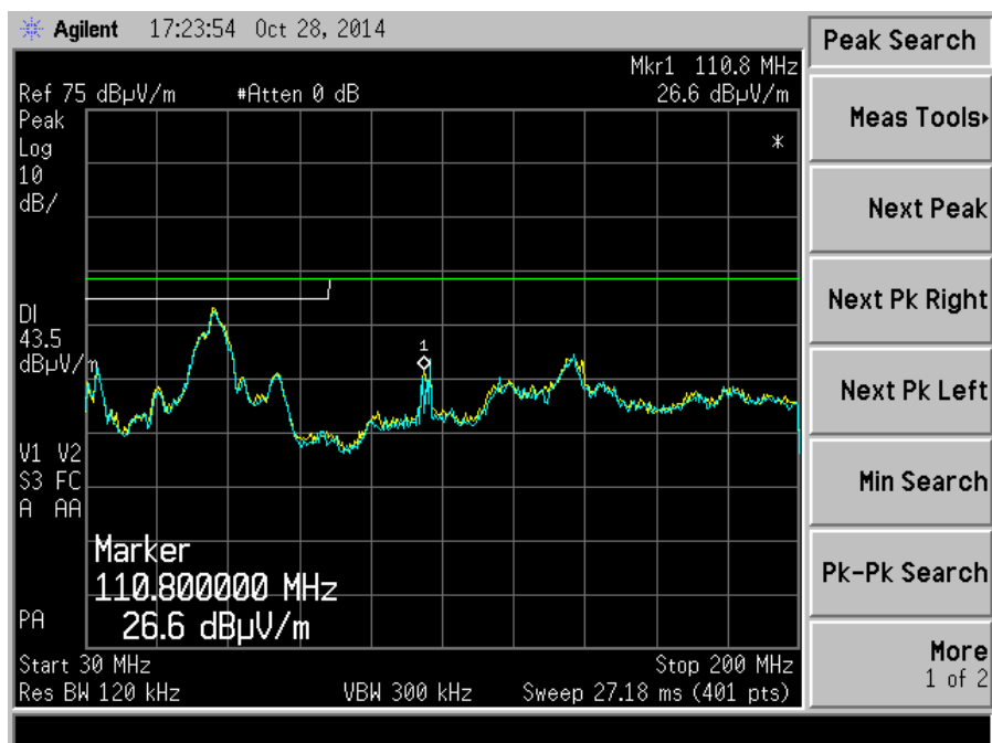
FIGURE 8: Radiated Emissions – Biconical, Horizontal Polarization Blue trace = EUT off, Yellow trace = EUT on
