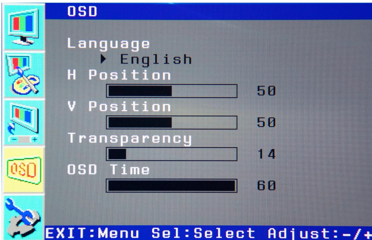
With the highlight in the fourth box from the top on the left, press the **SELECT** button to enter the OSD submenu.
