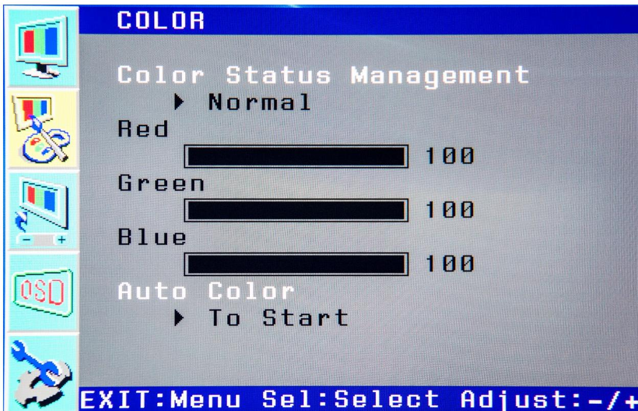
With the highlight in the second box from the top on the left, press the **SELECT** button to enter the Color submenu.
