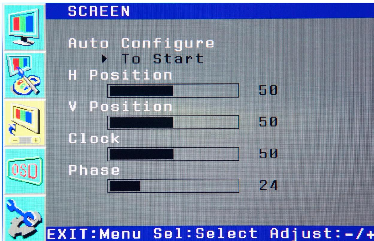
*Note that this screen is only available when using the RGB/VGA video input.*
