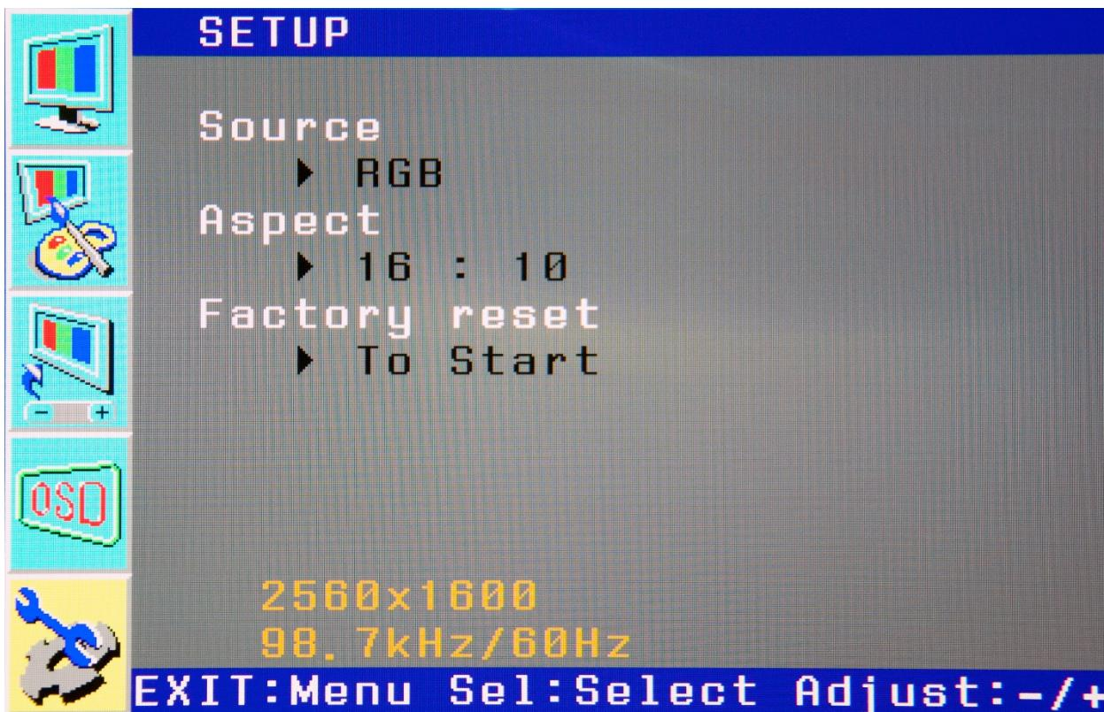
With the highlight in the bottom box on the left, press the **SELECT** button to enter the Setup submenu.
