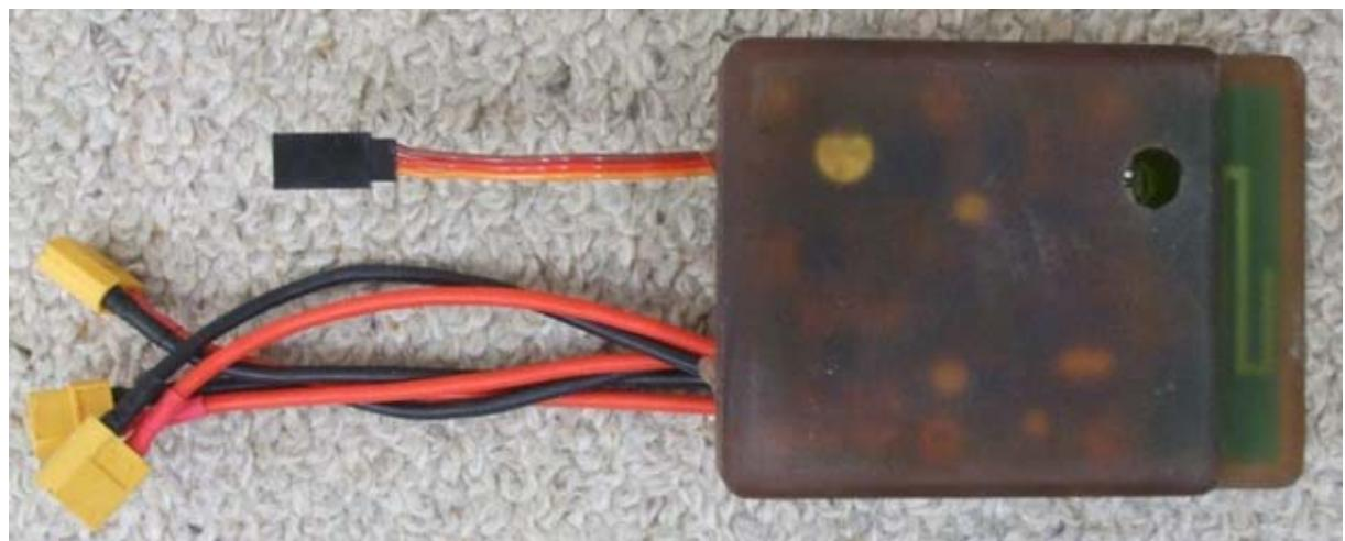
The antenna is located in the top quarter of the darker green portion of the circuit board directly below this writing
