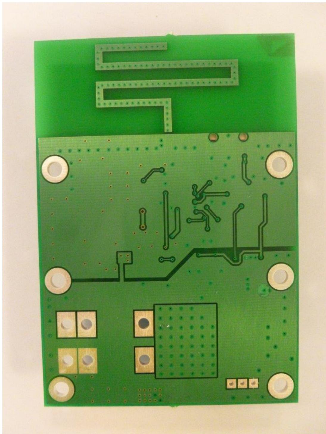
The antenna is located in the top quarter of the darker green portion of the circuit board directly below this writing.
