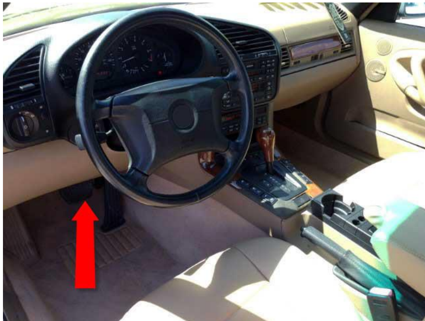
Figure 1-5: Common OBD-2 port location
