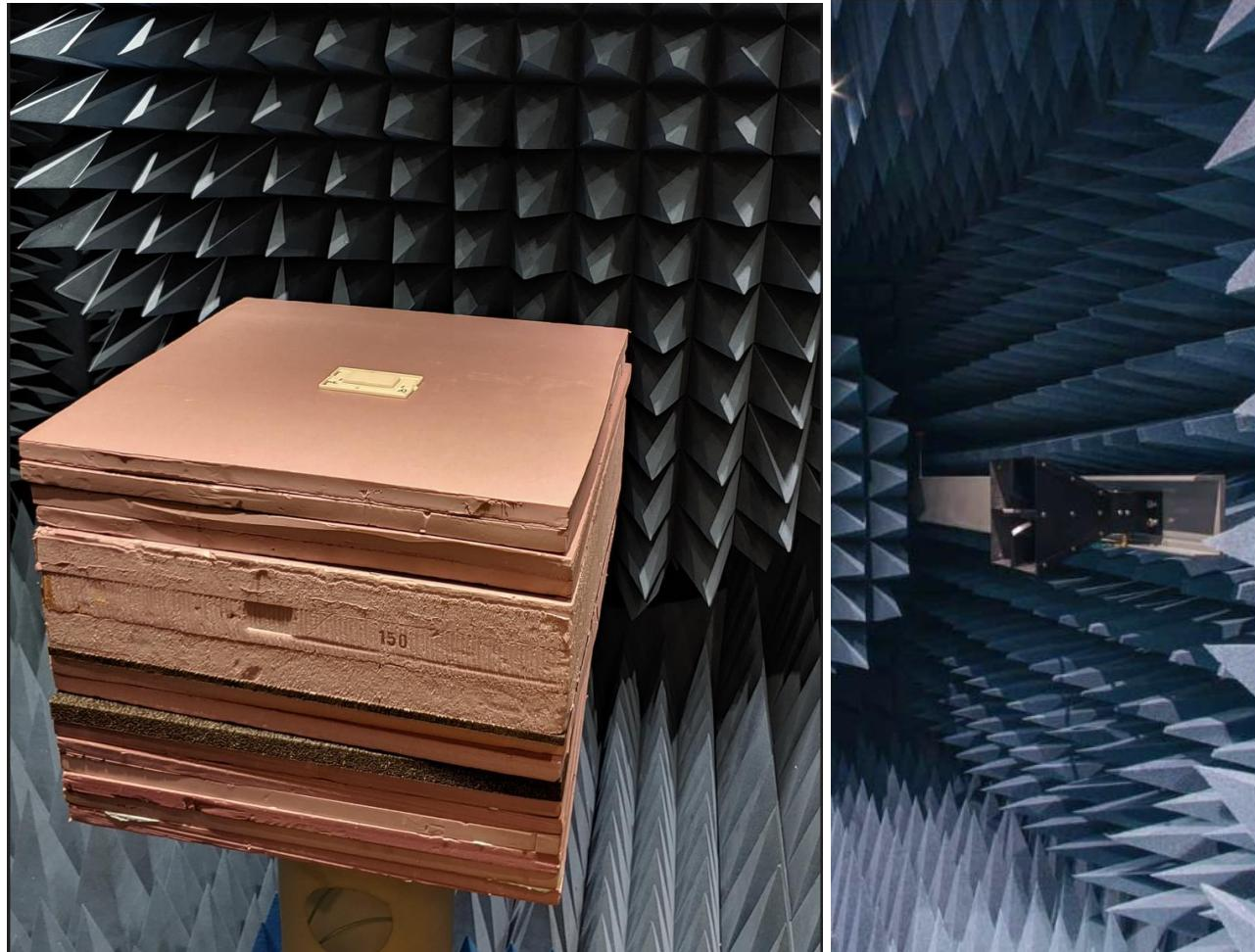
The first channel of the power sensor measures the vertical polarization of the dual polarized ridge horn, while the second channel measures the horizontal polarization.
