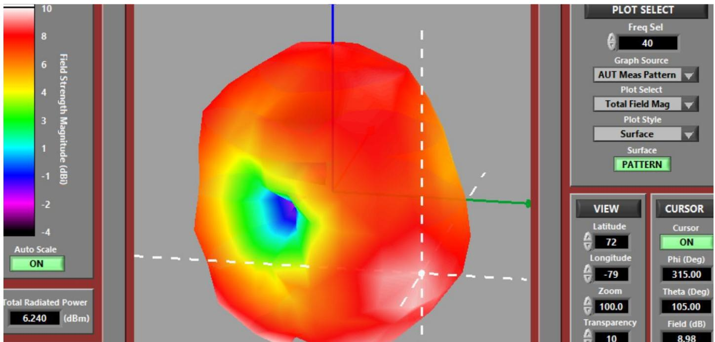
Radiation pattern for 2442 MHz IFA antenna. The peak gain at the cursor is  $8.98 - 6.24 = 2.74$  dBi
