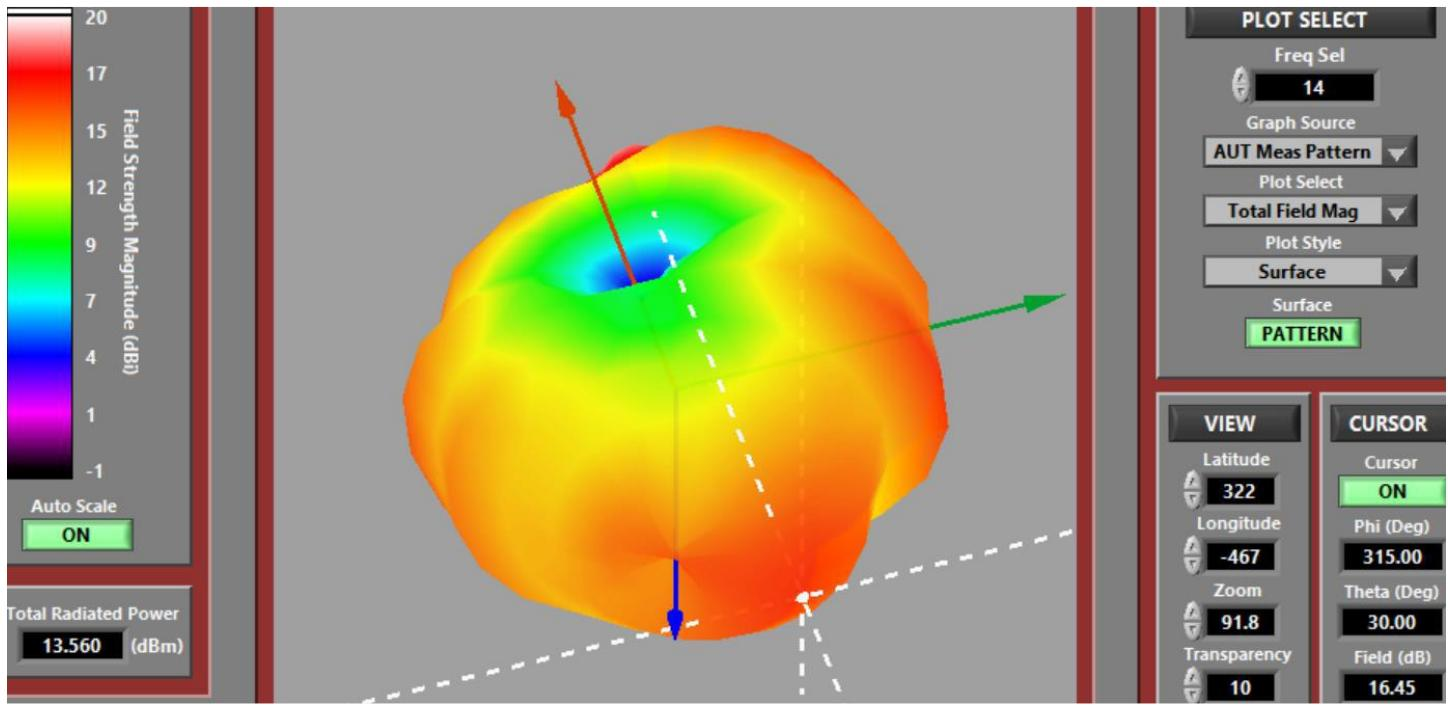
Radiation pattern for 914 MHz meandered dipole. The peak gain at the cursor is  $16.45 - 13.56 = 2.89$  dBi
