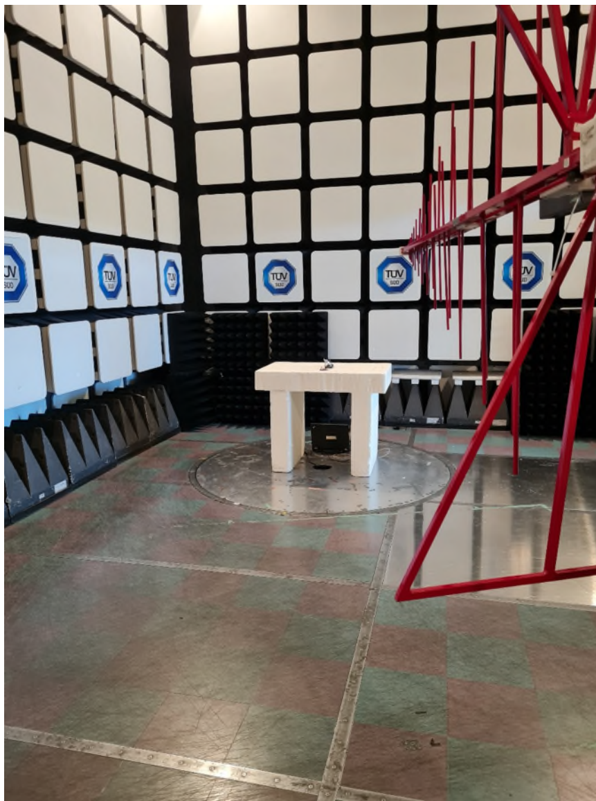
Figure 3 – Radiated Emissions Setup
