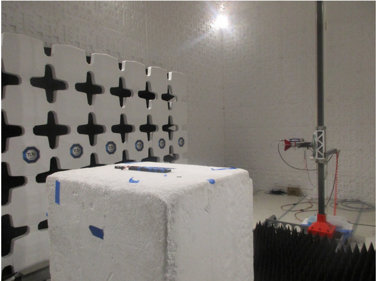
Figure 18: Radiated Emissions – Back View – External Flag Antenna
