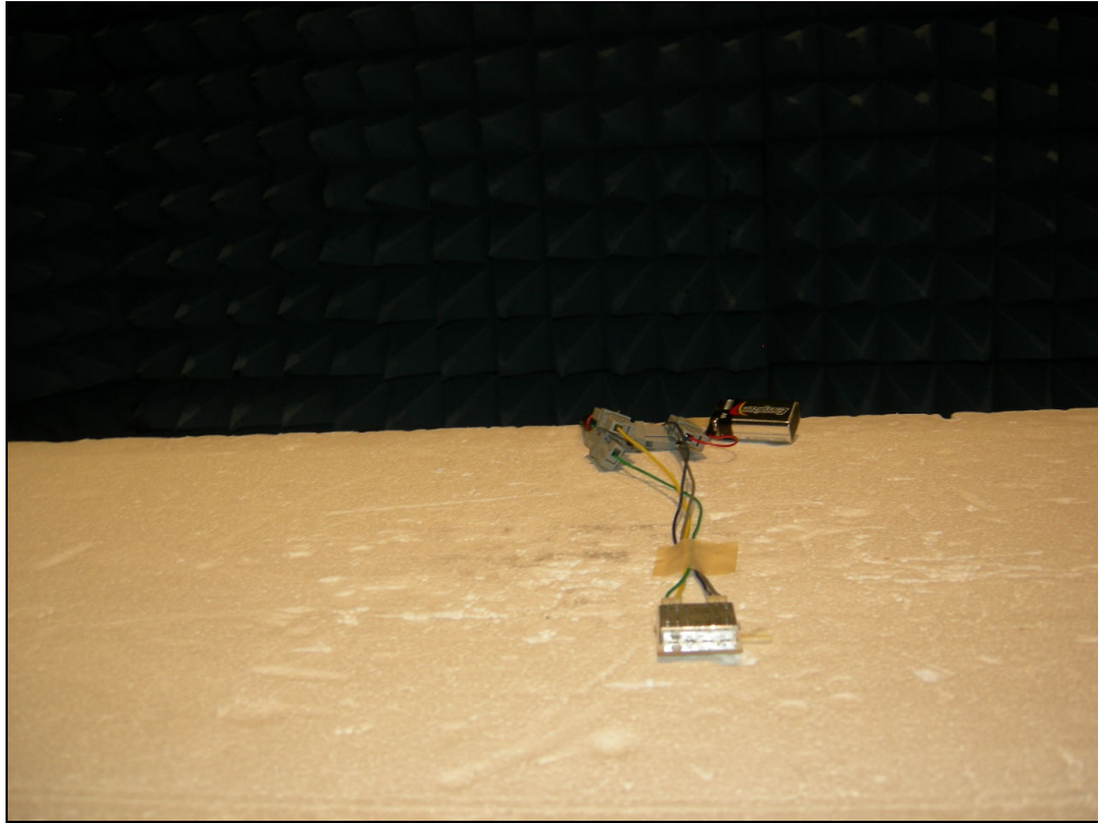
Figure 1: Radiated Emissions – Internal (Chip) Antenna – XPOS
