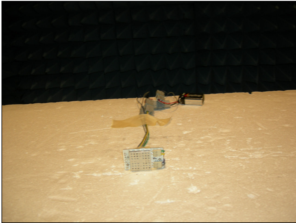
Figure 5: Radiated Emissions – Internal (Chip) Antenna – ZPOS
