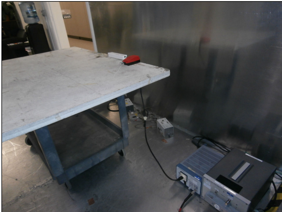
Figure 16: Conducted Emissions - External (PIFA) Antenna
