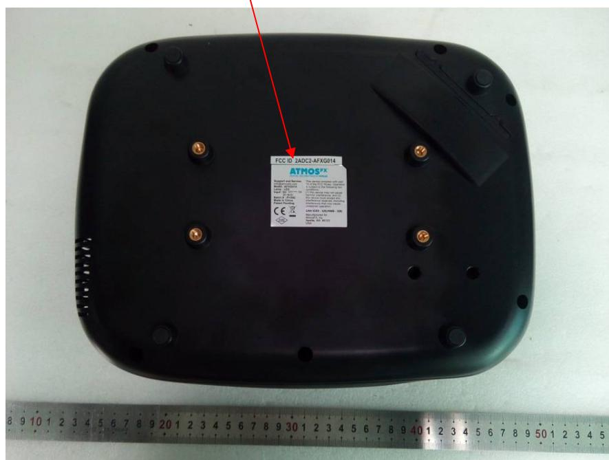
The label shown shall be permanently affixed at a conspicuous location on the device and be readily visible to the user at the time purchase (Labeling requirements per 2.925)
