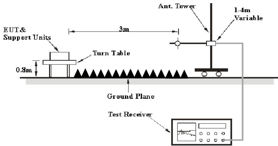
The radiated emission test was performed in the 3 meters chamber test site, using the setup accordance with the ANSI C63.4-2009. The specification used was the FCC Part 15.109, Class B limits.
