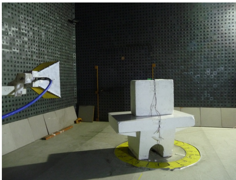
Photograph 8.1.2 Setup for radiated emission measurements
