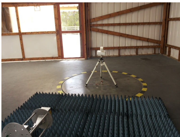
Photograph 8.1.4 Setup for final radiated emission measurements at the OATS
