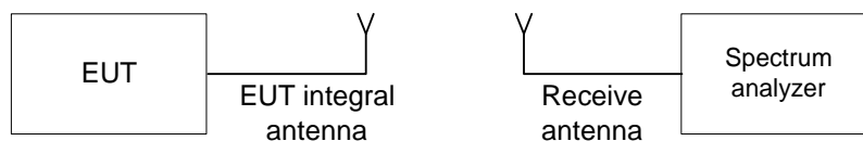
Figure 7.5.1 Setup for transmitter shut down test
