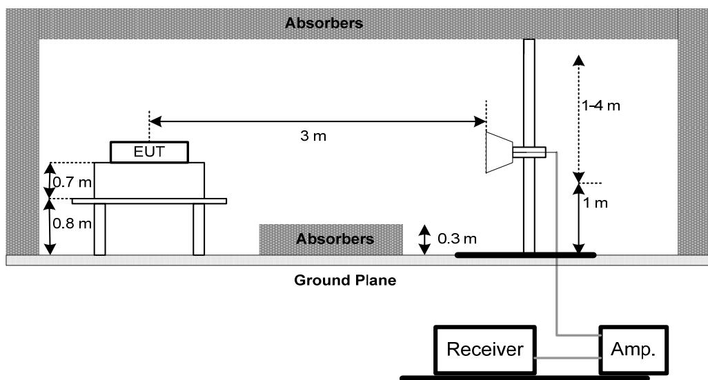
(C) For Radiated Emissions Below 30MHz
