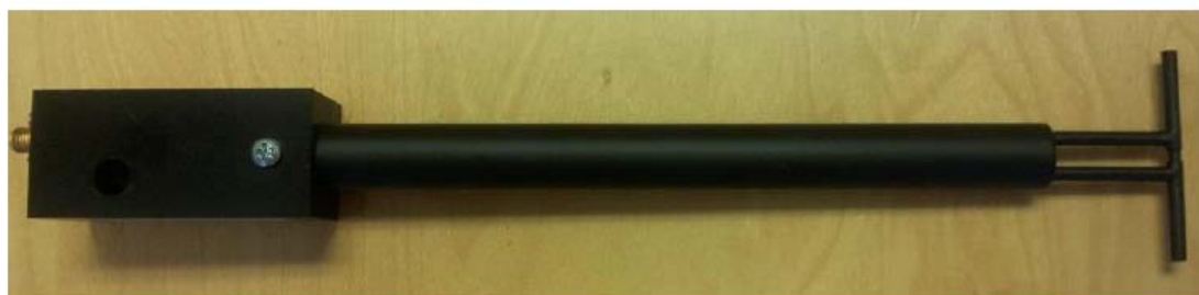
Figure 1 – MVG COMOSAR Validation Dipole
