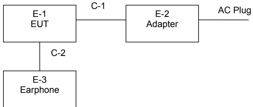
Radiated Spurious Emission Test
