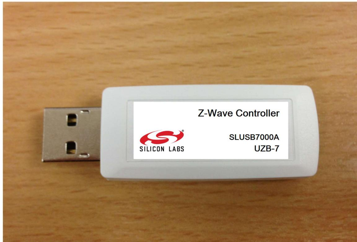
The dimension of the WHITE Sticker is **34mm x 12.5mm**. The material (white polypropylene) is splash proof adhesive type.
