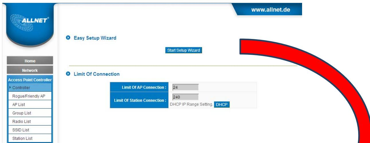
The Easy Setup Wizard feature in Access Point Controller helps user use several simple steps to configure Local AP. Follow the wizard to enter the SSID and password that you want.
