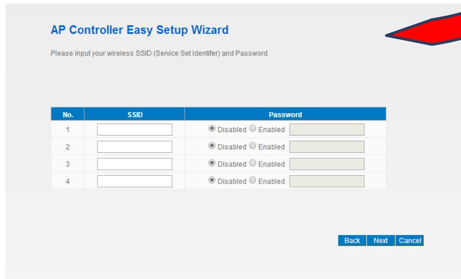
When you finished the Easy Setup Wizard, access point will restart automatically to commit the settings and the access point will apply the wireless settings.
