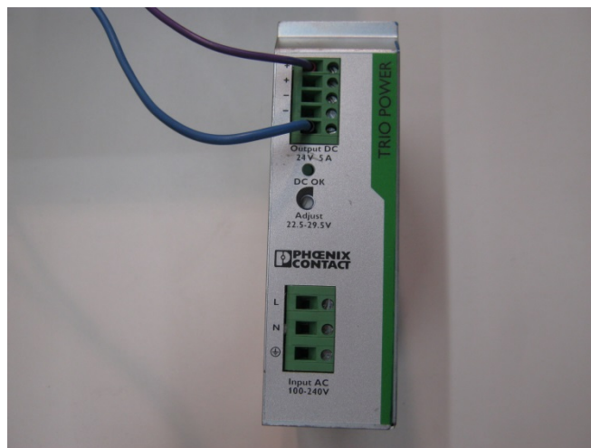
Photograph 2.3-2: Power supply TRIO-PS/1AC/24DC/5, front view
