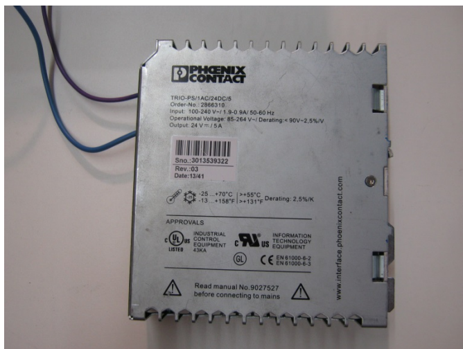
Photograph 2.3-1: Power supply TRIO-PS/1AC/24DC/5
