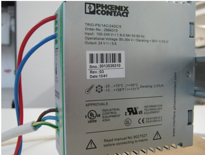
Photograph 2.3-1: Power supply TRIO-PS/1AC/24DC/5
