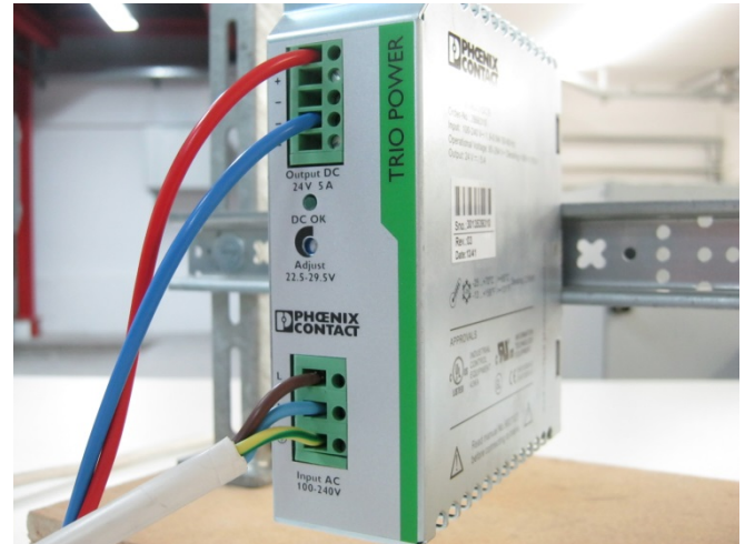
Photograph 2.3-2: Power supply TRIO-PS/1AC/24DC/5, front view
