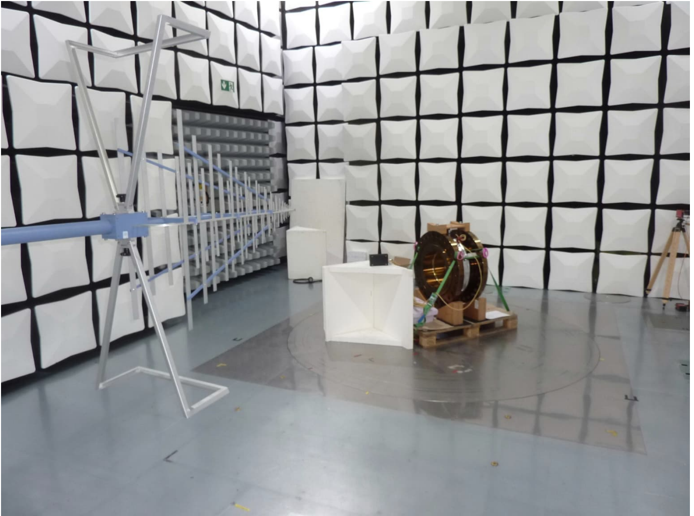
Setup 30 MHz to 1000 MHz radiated field strength measurement
