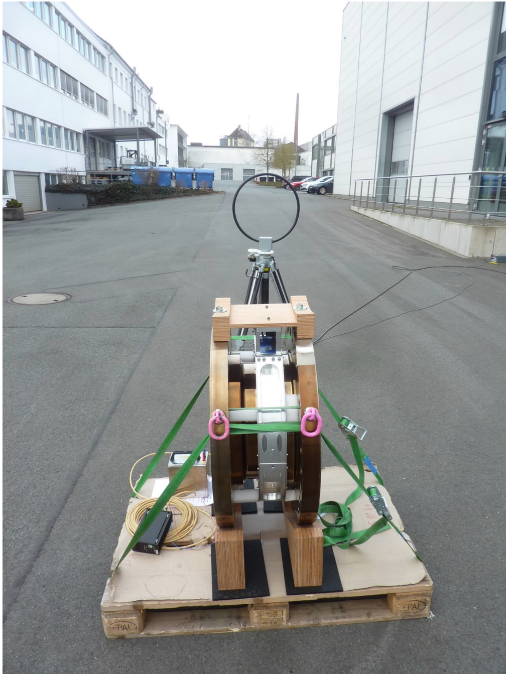
Setup 9 kHz to 30 MHz magnetic field strength final measurement
