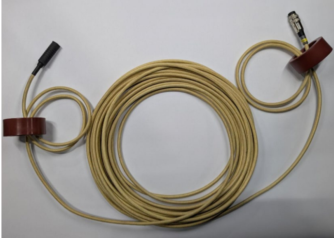
Fig 6.2: Picture of installation example of EMI suppressors
