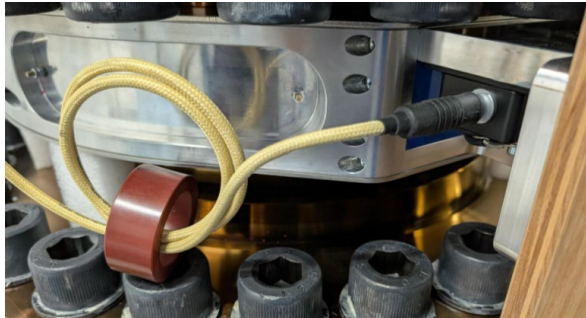
Fig. 4.3: EMI suppressor at stator unit
