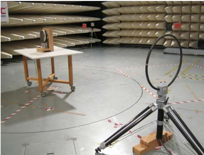
Radiated emissions measurement at 3 m distance 9 kHz – 30 MHz
