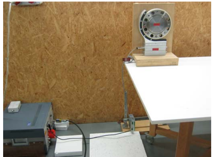
Conducted emissions measurement 9 kHz – 30 MHz
