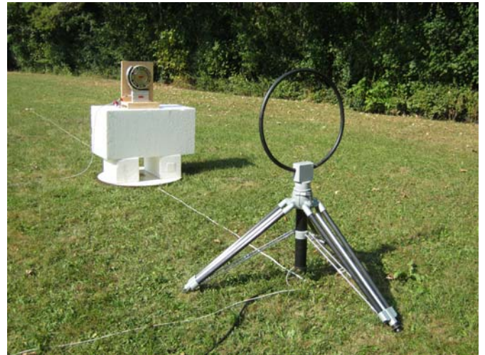
Radiated emissions measurement at 3 m distance at open area test site 9 kHz – 30 MHz
