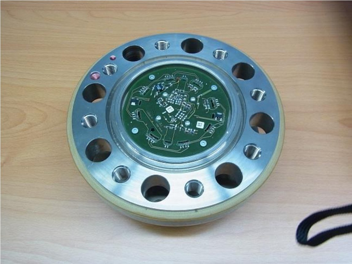
The rotor includes 4 PCB
