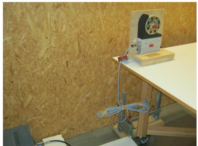
Conducted emissions measurement 9 kHz – 30 MHz
