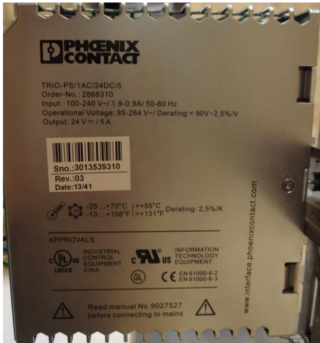
Photograph 2.3-1: Power supply TRIO-PS/1AC/24DC/5
