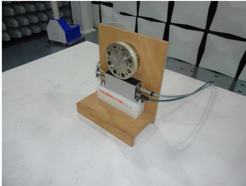
Test setup semi anechoic chamber (position 1)
