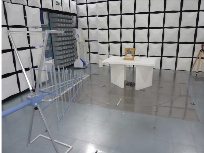
Test setup semi anechoic chamber (<1 GHz)
