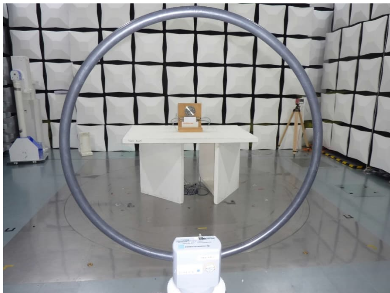
Test setup semi anechoic chamber (<30 MHz)
