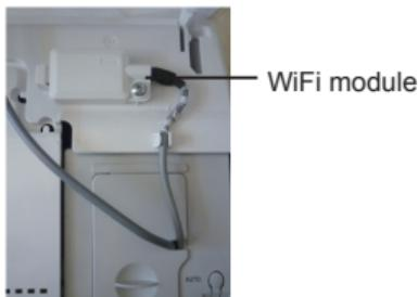
5. Neaten the WiFi connection wire, close the electric box cover and then tighten the screws.
