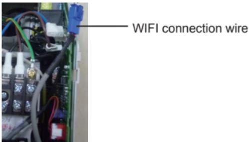
3. Pull out the WIFI connection wire from the electric box and then connect it with the port in WiFi module.
