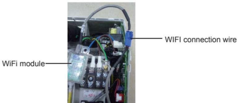
4. Place the WiFi module beside the electric box. After confirming the position, please fix the WiFi module with screws.
