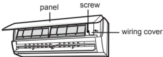
2. Open the electric box cover and you can see the WiFi connection wire. (The color of WiFi connection wire is the same as the color of connection port in WiFi module).
