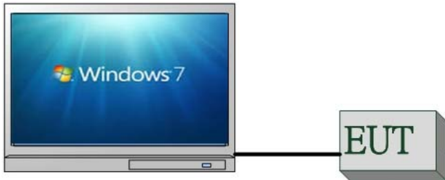
Fig. 2-1 Conducted (Antenna Port) Emission Configuration
