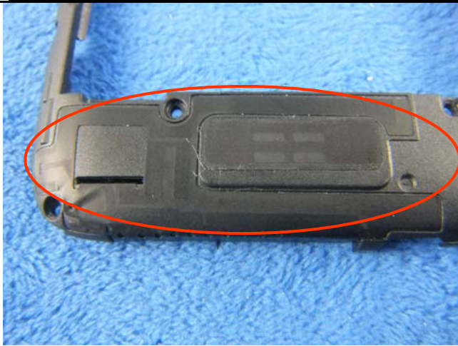
GSM/PCS/UMTS-FDD Antenna View
