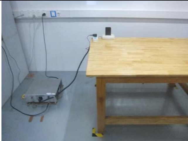
Conducted Emissions Test Setup Front View
