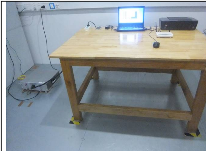
Conducted Emissions Test Setup – Front View
