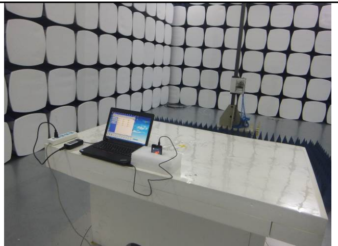
Radiated Spurious Emissions Test Setup Above 1GHz
