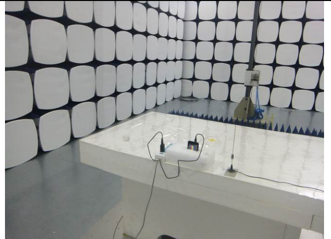
Radiated Spurious Emissions Test Setup Above 1GHz
